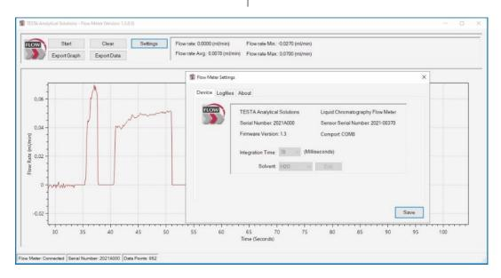
In fact, such non-invasive flowmeters are being evaluated to become a permanent component of HPLC/UHPLC systems delivering flow data directly to a Chromatography Data System along with all other detectors present, thereby enabling continuous validation of flow.
